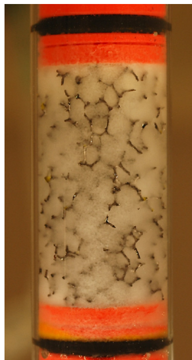
Fig. 5. Close-up of a glass column with an RVC–Cytopore composite. The dimensions of the composite are 25 mm × 10 mm (1 × I.D.). The RVC structure in immediate vicinity of the glass wall is clearly visible. The banded structures at the top and at the bottom of the column belong to the flow adaptors.
